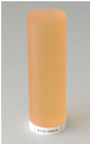
Bead phantom tungsten bead 0.3mm dia.
