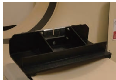
Phantom fixture of the scanner
